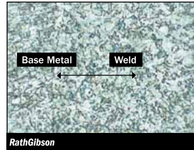
Optical image of RathGibson's 304L laser welded product with complete weld recrystallization. Note that the weld is virtually indistinguishable from the base metal.
