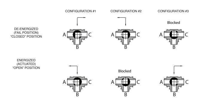
180° rotation actuators allowing for 2 or 3 position control are available upon request
