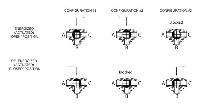
180° rotation actuators allowing for 2 or 3 position control are available upon request
