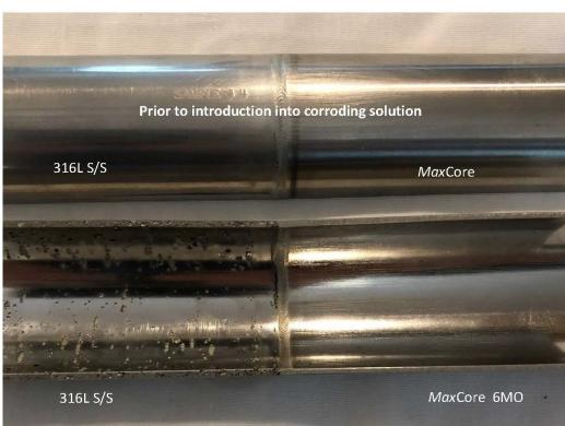
This picture shows a comparison of the corrosion resistance of 316L material vs. MaxCore 6Mo material. The materials were orbital welded together with no weld filler then put into a ASTM G-48 Practice C (modified immersion test) solution of 6%FeCl<sub>3</sub> + 1% HCl at 50° C (122° F) for 72 hours
